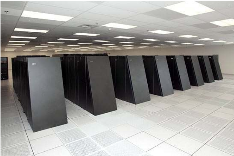
Blue Gene/P Supercomputer © 2009 IBM. 213,000 parallel PowerPC processors
